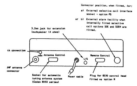
Fig. 1 Rear panel layout - Type 8525 B
