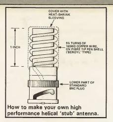
laboratory equipment, when mounted on a Yaesu FT708R, it was found to outperform the supplied 1/4 wave whip by 0.6dB! Excellent results are also given on the PF5UH and PF2UH. A number are in use by several amateurs in my locality.
