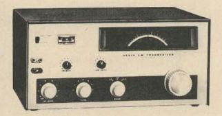
Bandswitching is in one front-panel switch and transmitter tuning is simple. All you do is dip the final plate current reading on the front panel meter—or peak the power output reading on the meter, whichever you choose. There is a power level control on the front panel which lets you vary the screen voltage on the 6GE5 final, raising or lowering the input power of the transmitter. That way you can stay within Novice limits or boost the rig's input to over 100 watts.
