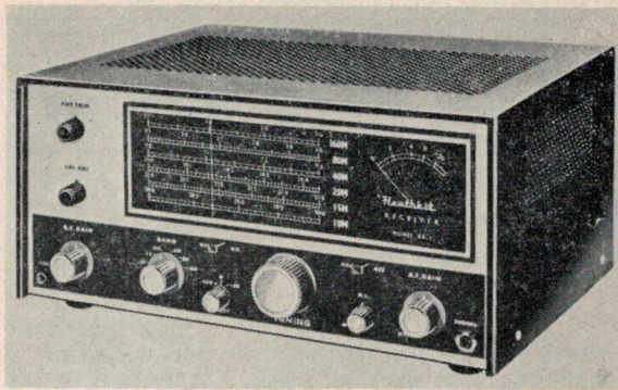
The Heathkit Model RA-1 amateur bands receiver. The cabinet is finished in silver and green. The panel controls (reading from the top left) are aerial trimmer, calibration adjustment, r.f. gain, band-switch, b.f.o. on/off, sideband selection switch, main tuning, a.v.c. on/off, noise limiter and a.f. gain. The phones jack is at the bottom right-hand corner of the front panel.
