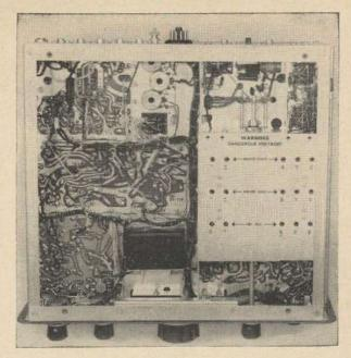
cuit boards, each with a switch wafer and associated components, that is used for the bandswitch.
