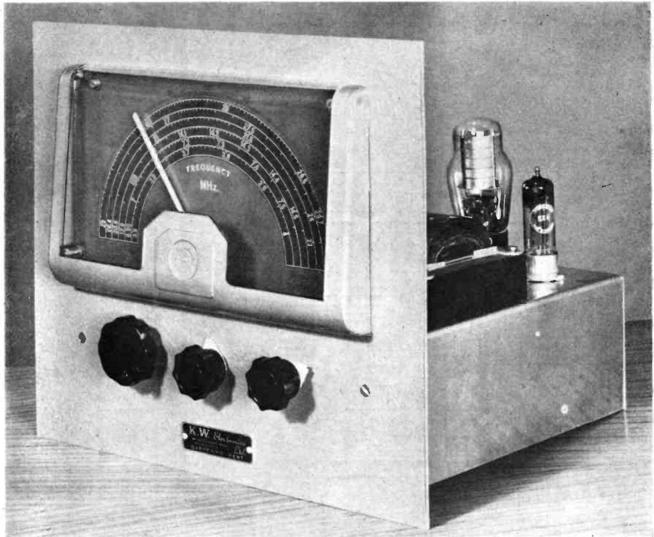
General appearance of the Geloso Receiver Front End, which makes up as a self-contained unit, the circuit being as shown in Fig. 1. Full spread is given across all amateur bands, including the 27 mc (11-metre) band as a separate range, and the Converter will work into any receiver tunable around 4.6 mc as the IF/AF amplifier. It will improve considerably the HF-band performance of most receivers, and is easy to assemble and instal.
